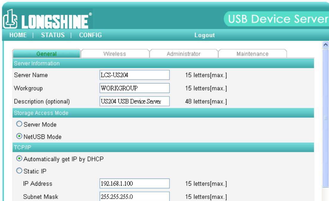
Figure 3 TCP/IP Setting
